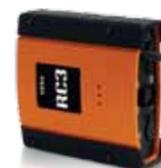
**RC3**, on the other hand, in addition to the two modes offered by RC2, reads the values directly from the OBD socket (using EOBD protocol), thereby allowing for the test to be performed, without even having to open the bonnet.
